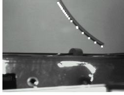
Figure 7: With the stationary camera detected pneumatic wire and found base points (white dots)
