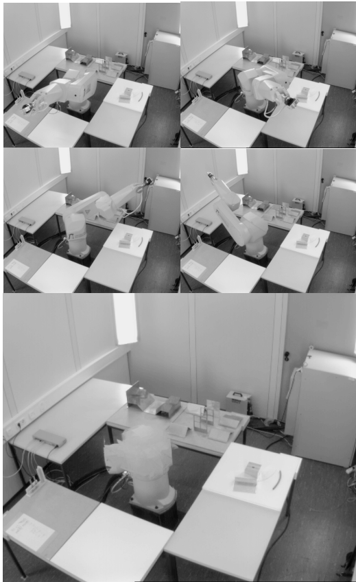
Figure 7: Reference Image Creation. The four smaller images are acquired by the camera. Together with five other pictures showing the robot in different configurations, the reference grayscale image is created. The result using the median of all nine images is shown in the larger image.
