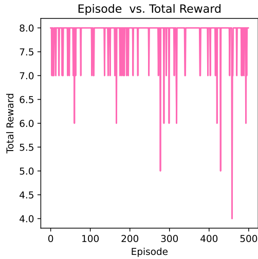
Figure 6.39: Episode versus total reward for the double Q -learning agent with the function approximation method
