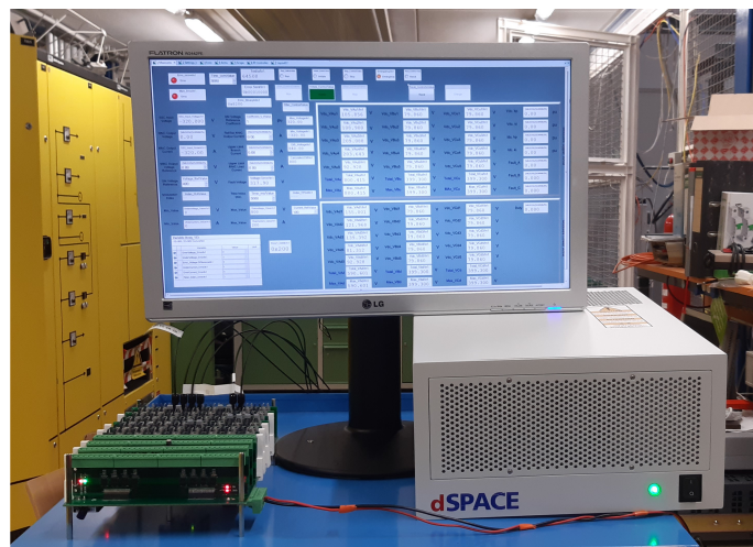
Figure 5.10: Control platform – dSPACE , central FPGA and user interface
