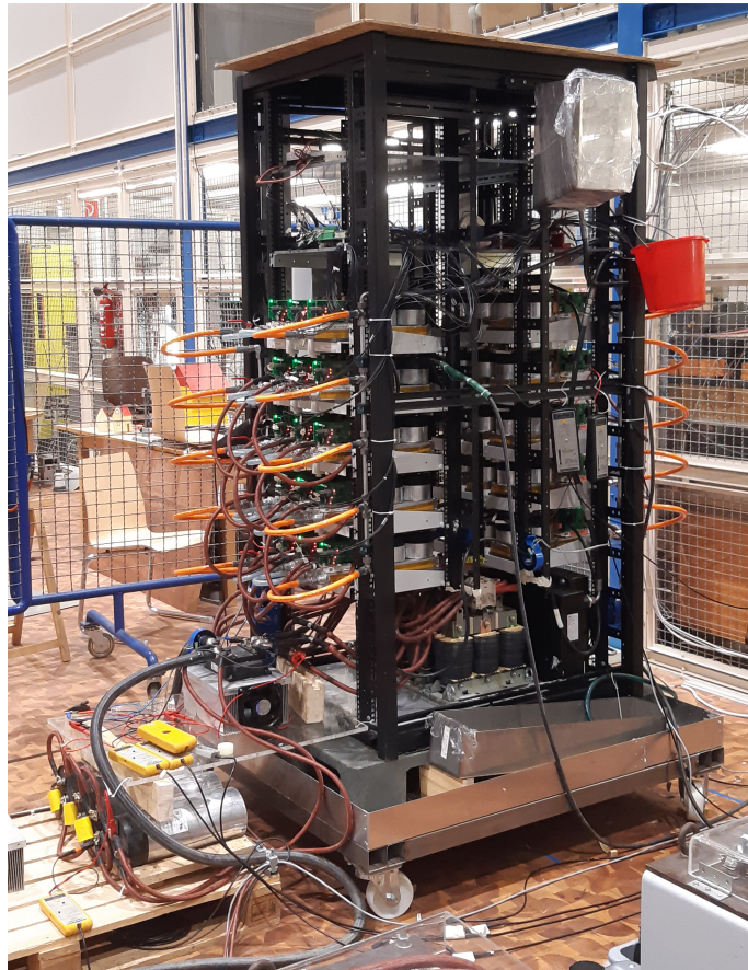
Figure 5.8: Mobile Side Converter – 300 kW Demonstrator
