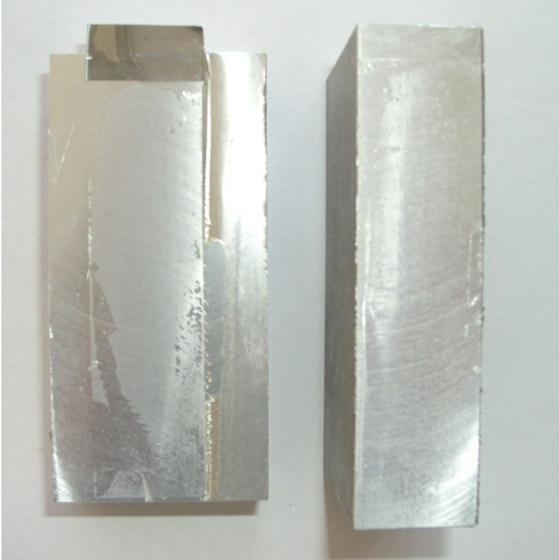
Fig. 3.10 Photo of the aluminum plates bonded by the Araldit LX 3505 glue
