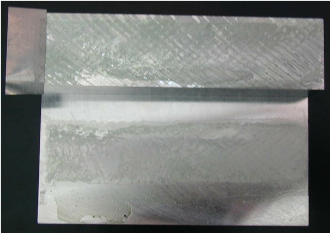
Fig. 3.6 Photo of The Aluminum Plates Bonded by the Loctite product 603 glue
