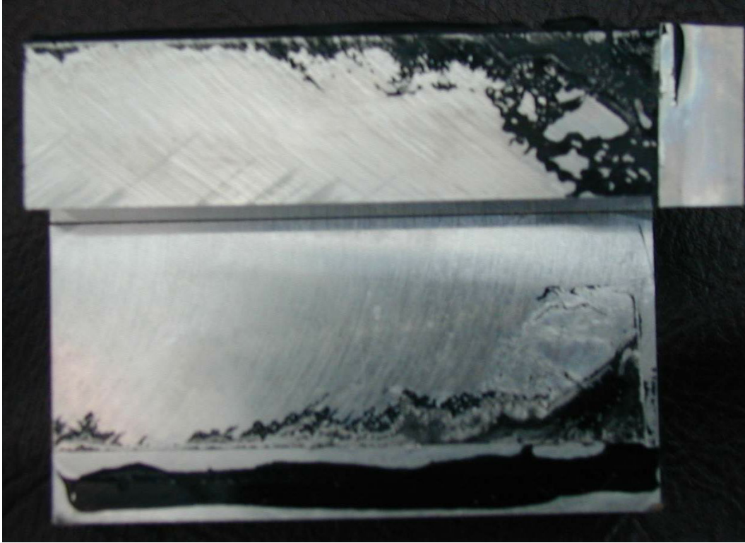
Fig. 3.3 Photo of The Aluminum Plates Bonded by the Loctite product 480 glue
