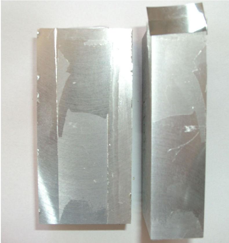
Fig. 3.11 Photo of the aluminum plates bonded by the Araldit 2020 glue
