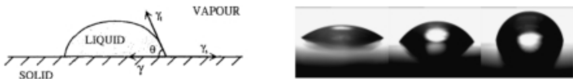
Fig. 3: Determination of surface energy by sessile drop contact angle measurement. The measured contact angle \theta is the angle between the drop base line and the tangent to the drop profile in the three phase point as shown in the left figure ( \gamma_L is the surface tension of the liquid, \gamma_S is the surface tension of the solid). The right three pictures show water drops on different solid surfaces varying in their surface energy from hydrophilic to hydrophobic (left to right). Taken from [1, 2].
