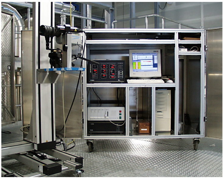
Figure 3: Test stand for velocity and temperature measurement: Infrared Camera and Laser Doppler Anemometer
