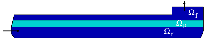
Fig. 3. A schematic drawing of a vertical cross-section of the filter
