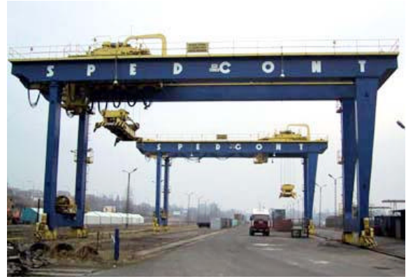
Figure 3: RMGC in the Krakow Krzeslawice Container Terminal, Poland
