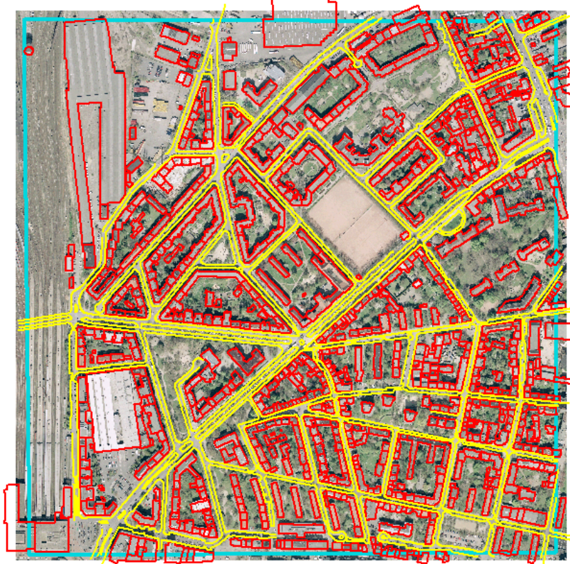
Figure 12: Subarea of Ham- burg-St. Pauli of size 1 km x 1 km. Input to the model build- ing are – in addition to the laser-scan points (see Figure 14) – polygons describing houses and compounds of houses (red), poly- gons describing curbs (yellow), and the outer border (blue).
