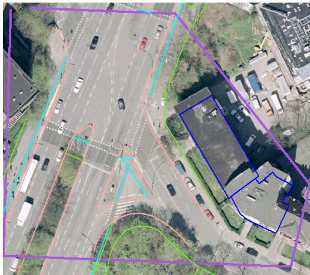
Figure 9: Photo and constrain- ing polygons for test 2; border of the area (purple), house boundary (blue), curb lines (pink), footpath borders (green), bicycle path (light blue).
