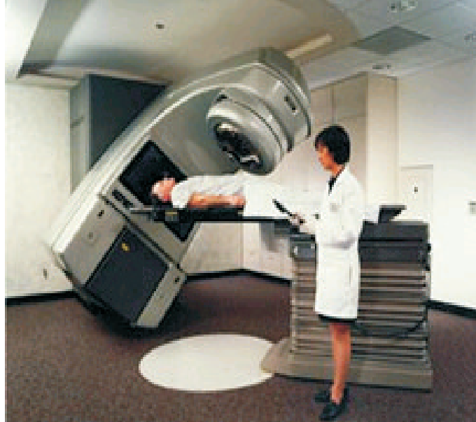
Figure 1.1: A medical linear accelerator with beam head and a couch. A patient is being treated.
