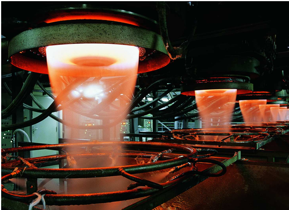
Figure 1.2: Glass wool production in a centrifugal spinning process.
