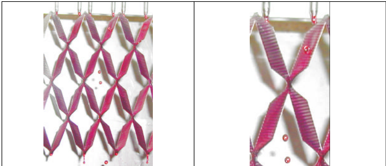
Figure (4-13): Liquid flow pattern for chlorbenzene – ethylbenzene 50% (16.9 ml/min.plate) with capillaries locate about 10 mm distance apart from the plates surfaces
