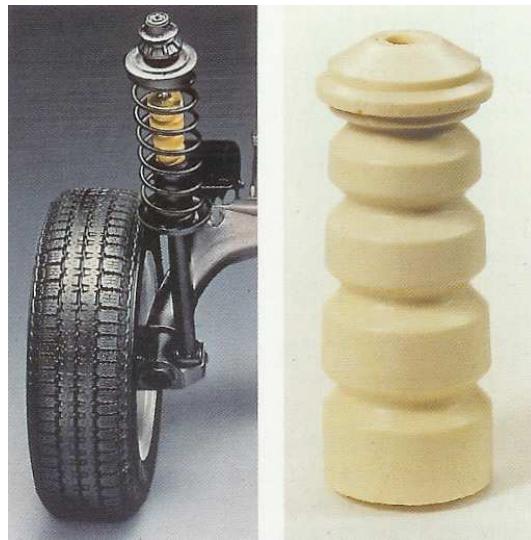
Figure 7.11: Spring aid in a spring leg (Elastogran GmbH). Photo taken from R. Leppkes [33] by permission of Verlag Moderne Industrie.
