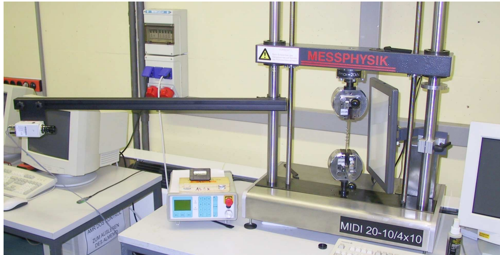
Figure 7.2: CCD camera for video extensometry in a tensile test.
