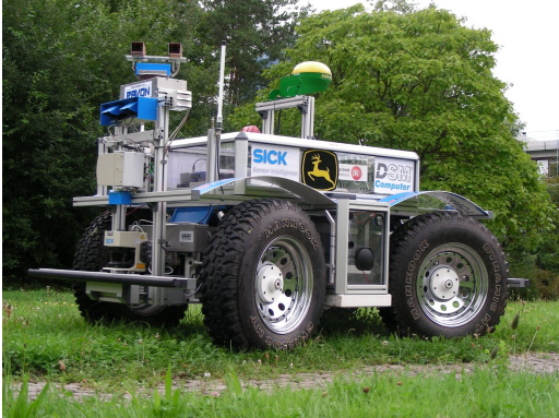
Figure 1.1: Robust Autonomous Vehicle for Off-road Navigation (RAVON). Research platform for behavior based motion, localization, and navigation strategies in rough terrain. Equipped with two stereo vision heads.
