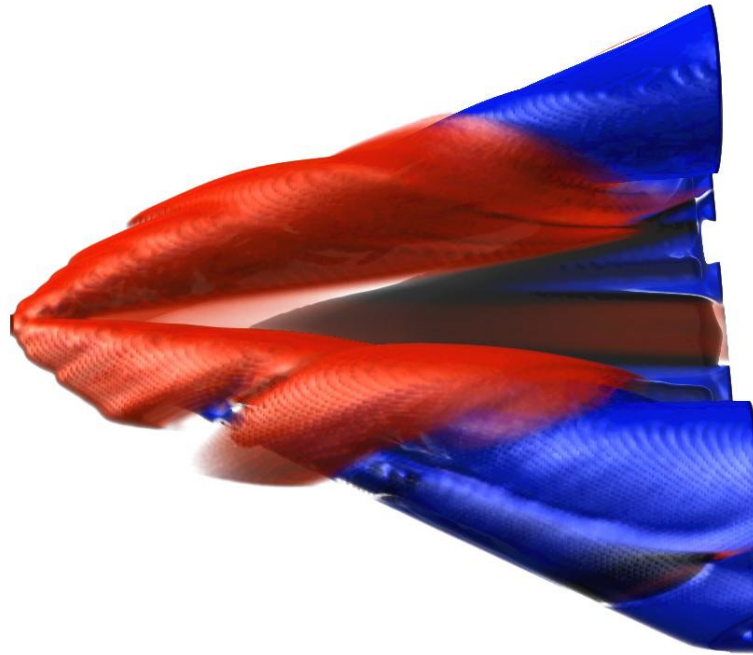
Figure 5.10: Volume Rendering of \sigma_n^+ \times \sigma_n^- (TDELTA). Wing edge separation and the primary attachment layer. Occlusion is problematic and has to be resolved through the use of cropping or clipping (Figure 5.11).
