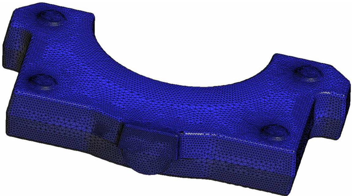
Figure 5.5. Surface mesh representing the shape of the bearing cap.
