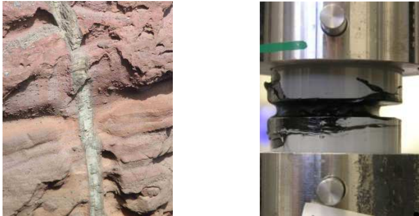
Figure 1.1: Example for a material interfaces within a bulk material of different properties: Rock with material layer of different properties; circular polyurethane tensile-test specimen, semi-cured (courtesy of Gunnar Possart).
