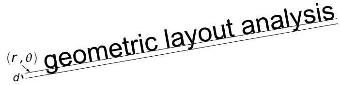
Figure 6.2: An illustration of Roman script text-line model proposed by Breuel [Bre02b]. The baseline is modeled as a straight line with parameters (r, \theta) , and the descender line is modeled as a line parallel to the baseline at a distance d below the baseline.
