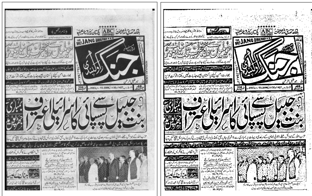
Figure 6.11: An example image cropped from the front page of a newspaper containing both normal and inverted text in the same image. The binarization step fails to identify the inverted text and makes it a part of the page background (white) as shown in the binarized image. (cp. [SuHKB06])
