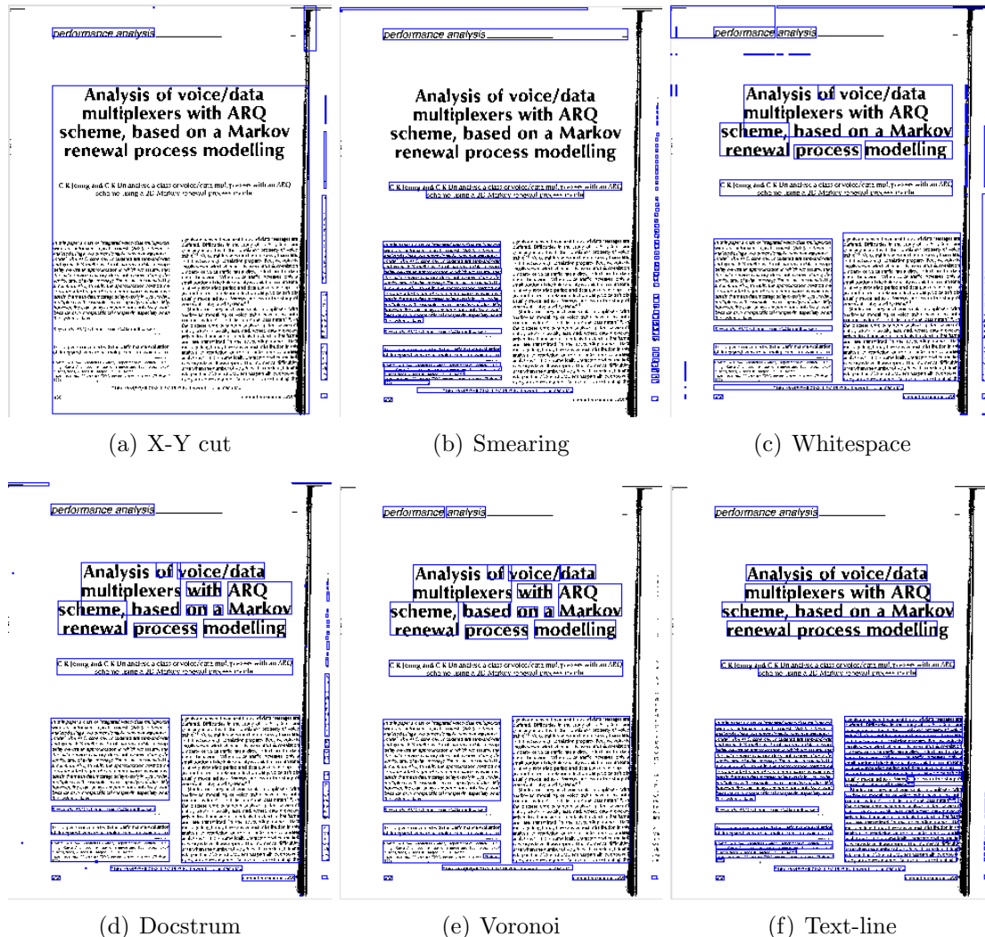
Figure 4.10: Segmentation results from applying each algorithm to one page image. The page contains a title in large font and a big noise strip along the right border. (a) The x-y cut algorithm fails in the presence of noise and tends to take the whole page as one segment. (b) The smearing algorithm also classifies the detected regions as text/non-text, and thus misses the lines joined by the noise bar. (c),(d),(e) Due to the large font size and big inter-word spacing, the Voronoi, docstrum, and whitespace algorithms split the title lines. (f) Due to the noise bar, several characters on the right side of each line in the second column were merged with the noise bar and the text-line finding algorithm did not include these characters. (cp. [SKB08b])
