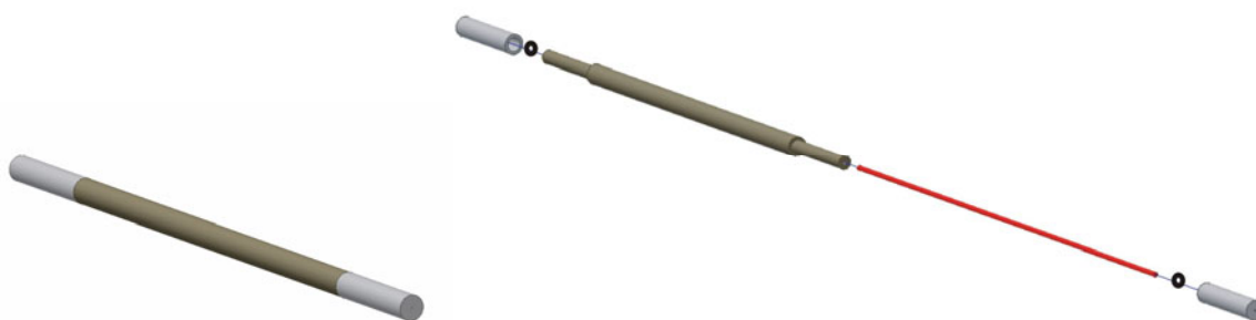
Figure 2.3: Scheme of the custom-built PEEK transfer capillary (3D scheme by H. Kampschulte).
