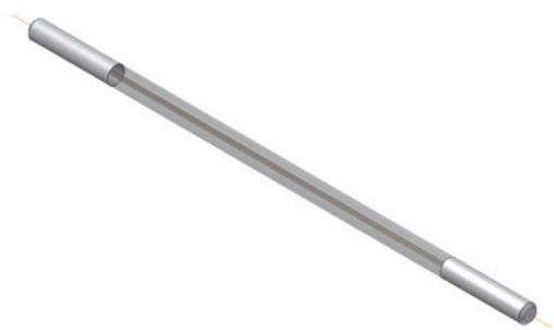
Figure 2.2: Scheme of the metal coated glass transfer capillary used in the Bruker Apollo I ESI source (3D scheme by H. Kampschulte).
