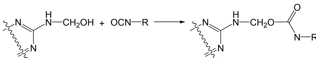
Fig. 2.1.29 – Reaction between melamine formaldehyde and isocyanate.
