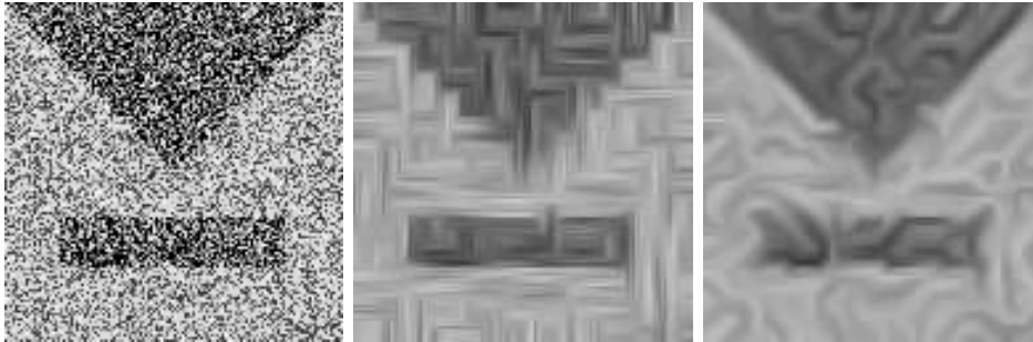
Figure 2: Sensitivity of sharp operator based anisotropic diffusion with respect to the number of directions. Left: Noisy input image, Middle: Sharp operator based diffusion with 2 directions, Right: Same with 4 directions.
