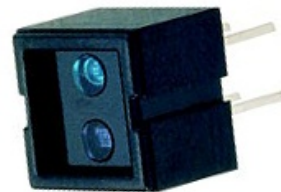
Figure 3.5.: CNY70 reflective optical sensor that is used for rotation speed detection.
