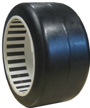
Figure 3.4.: One wheel with its attached black and white encoder strip.
