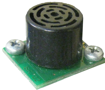
Figure 3.8.: Two of those SRF02 distance sensors are used for measuring the distance to the predecessor vehicle.
