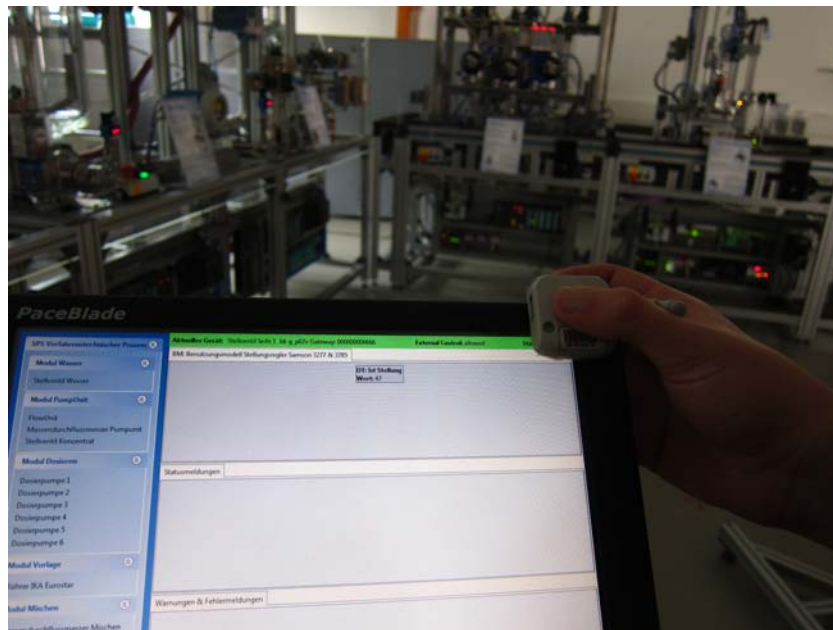
Figure 8.3.: The generated GUI shows read-only parameters. Setting parameters is disabled from the second zone.
