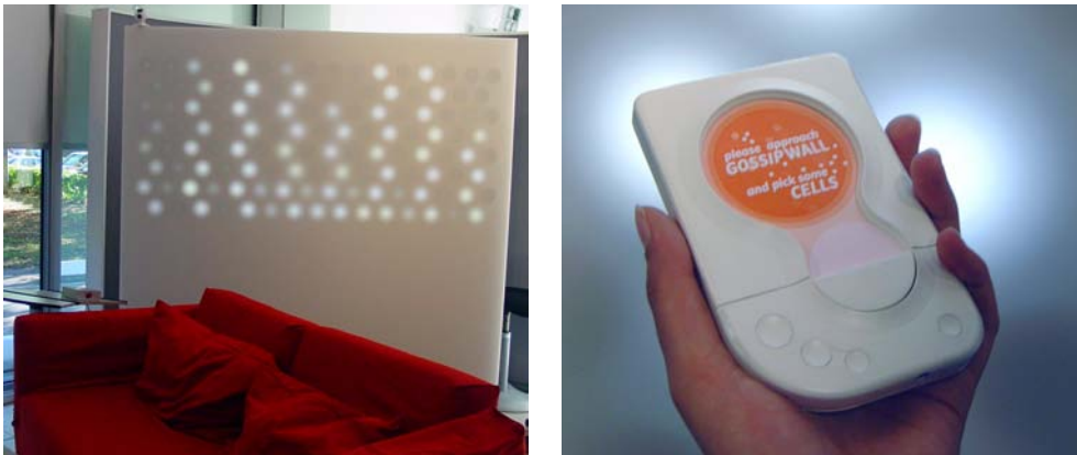
(a) Front-view of the Hello.Wall in ambient mode (b) The viewport used to interact with the wall
