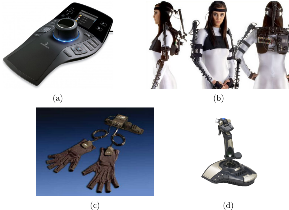
Figure 3.1: Examples of interaction devices for large high-resolution displays: (a) 3Dconnexion SpacePilot™ Pro [3dc] Image courtesy of 3Dconnexion Inc., Tobias Keuthen , (b) Animazoo Gypsy™ motion capture suit [ani] Image courtesy of Animazoo, Paul Collimore , (c) 5DT DataGlove Ultra Wireless™ [5DT], (d) Saitek Cyborg evo Force Feedback™ joystick [sai] Image courtesy of Saitek Inc.
