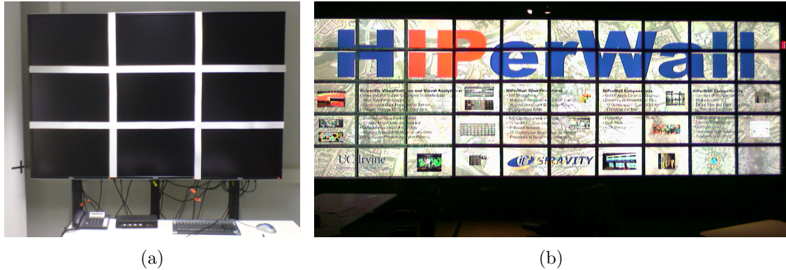
Figure 2.2: Tiled wall installations: (a) 3 \times 3 tiled display wall driven by 5 render nodes, (b) HIPerWall, a 200 megapixel 10 \times 5 display cluster driven by 25 render nodes.
