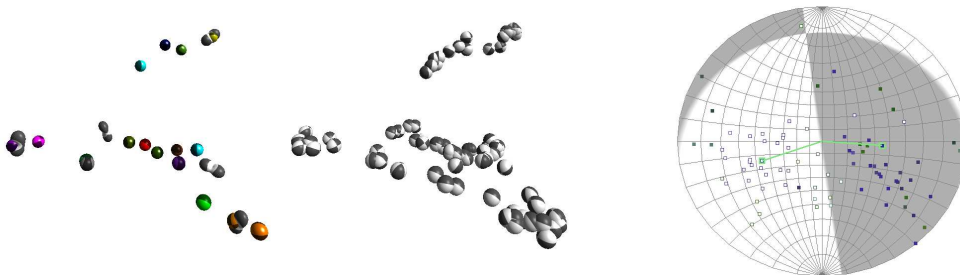
Figure 7.12.: Comparison of cluster averaging and polarity glyph display with classic unclustered beachball visualization (left). Moment tensor highlighting in stereonet view identifies related wave propagation directions and uses watermarking for fault plane orientation display (right).
