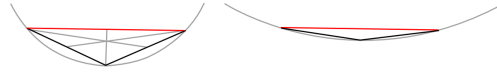
Figure 6.9.: Circumradius of the triangle adjacent to the boundary edge (red) increases after particle insertion, as the boundary edge cannot be flipped to produce better conditioned triangles. Such cases are avoided by splitting of boundary edges.
