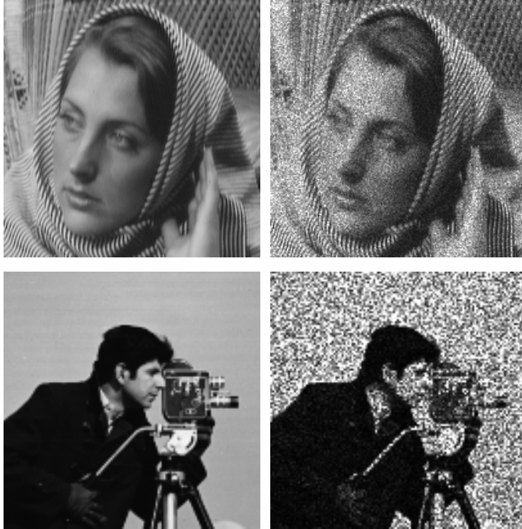
Figure 8: Left : Original images with values in [0, 255] . Right : Noisy versions corrupted by multiplicative Gamma noise with L = 25 (top) and L = 4 (bottom).
