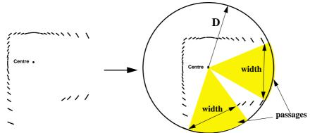
Figure 3:A Current Sensor Map and two passages at a distance D
