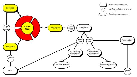
Figure 2: Control structure of MOBOT-IV
