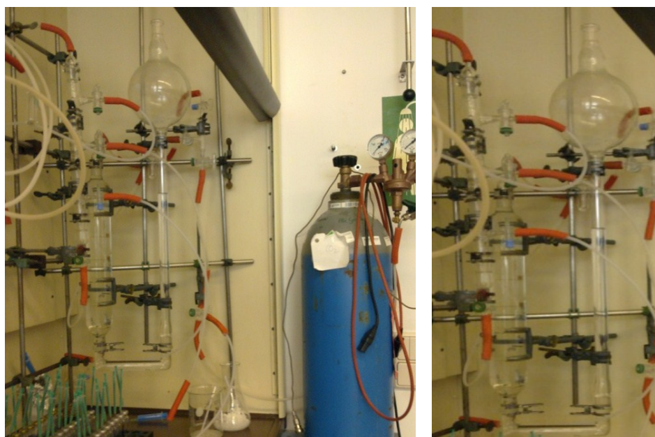
Figure 2. Modified reaction setup for carboxylation reactions: 1200 mL CO 2 glass container.
