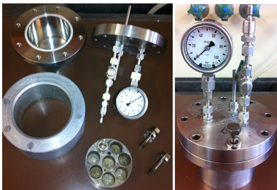
Figure 3. Autoclave-reactor manufactured by the Max-Planck-Institut für Kohlenforschung.
