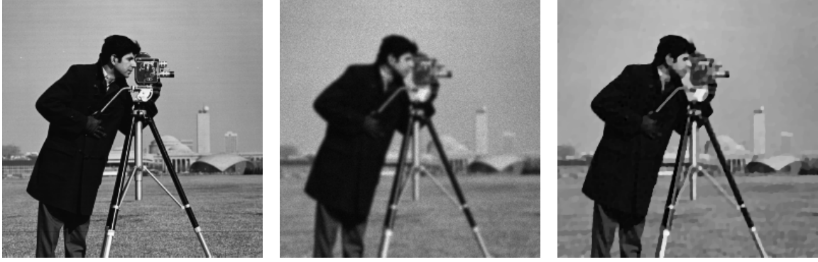
Figure 3.6: Left: Original 'cameraman' image of size 256 \times 256 . Middle: Image corrupted by a Gaussian blur (standard deviation \sigma = 1.3 ) and Poisson noise ( I_{\max} = 1000 ). Right: Deblurred image by IDIV-TV with \lambda = 0.01 .
