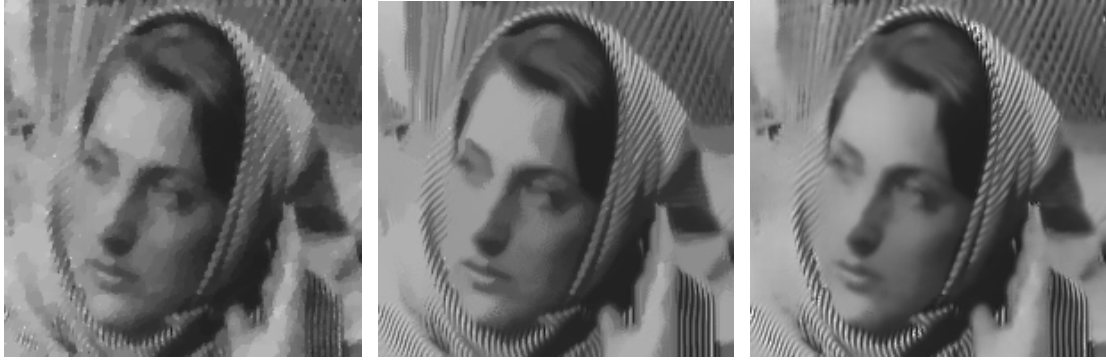
Figure 4.9: Results for the noisy image at Figure 4.8 (top right) by the IDIV-TV (left) and IDIV-NL model (middle) as shown in Figure 3.10 and a result by our nonlocal filter (4.27) using the weights (4.30) with l = 7 , \omega = 21 , a = 2.5 , h = 1 , q = 0.6 (right).
