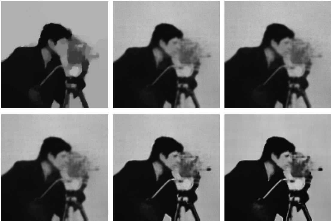
Figure 4.10: Results for the noisy image at Figure 4.8 (bottom right). Top : Restored images by IDIV-TV as presented in Figure 3.11 (left), by the original NL means filter using s_{NL}(\log(\cdot), \log(\cdot)) instead of s_{NL} with l = 7 , \omega = 29 , a = 1.5 , h = 1.3 (middle) and by our new nonlocal filter (4.27) using the weights (4.29) with l = 7 , \omega = 29 , a = 1.5 , h = 1 (right). Bottom : Results by our nonlocal filter using (4.30) with additional parameter q = 0 (left), q = 0.35 (middle) and finally after an additional updating step with \tilde{l} = 3 , \tilde{a} = 0.5 , d = 0.25 (right).
