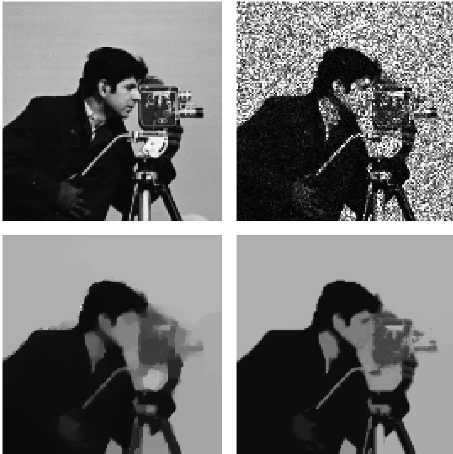
Figure 3.11: Top : Original image (left) and noisy version corrupted by multiplicative Gamma noise with L = 4 (right). Bottom : Restored image by IDIV-TV with \lambda = 0.9 (left) and the result by the IDIV-NL model with \lambda = 0.6 , l = 5 , \omega = 21 , a = 1.5 and \tilde{m} = 5 (right).
