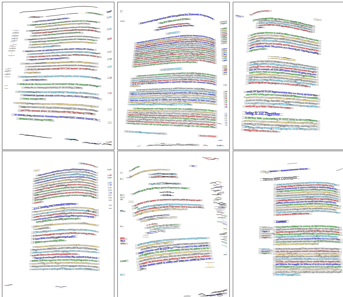
Figure 2.13: Accurate curled text line segmentation results of coupled snakelets algorithm for camera-captured document images of the DFKI-I dataset. [Note: text line segmentation results are shown in color coded form using repetition of six different colors. Two or more text lines with same color do not necessarily mean undersegmentation error. In order to avoid this confusion, coupled snakelets are also drawn here to mention the boundary of each segmented text line.]
