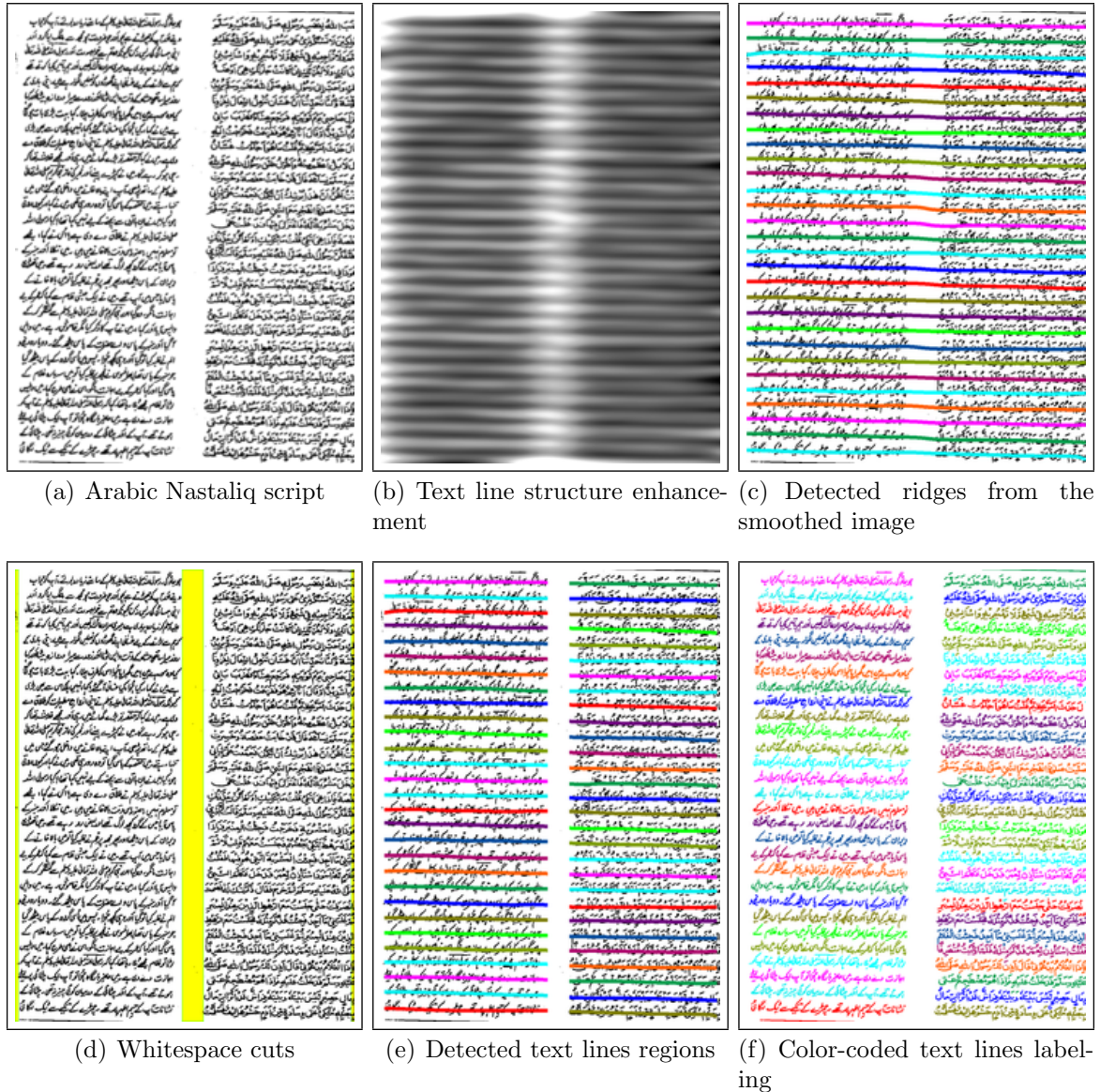
Figure 10.8: Steps of the ridge-based text line finding algorithm. a) An example image of Arabic Nastaliq script. b) Smoothed text lines (text lines enhanced) image, which is generated by using oriented anisotropic Gaussian smoothing filter bank approach. (c) Detected ridges from smoothed image using Riley based ridge detection [Ril87b, Ril87a] algorithm. There are over-segmentation errors because of multi-column. (d) Column separators that were detected through whitespace analysis; these separators help in correcting over-segmentation errors. (e) Processed ridges using whitespace separators; each ridge covers a complete region of a particular text lines. (f) Color-coded labeled text lines result using detected ridges.
