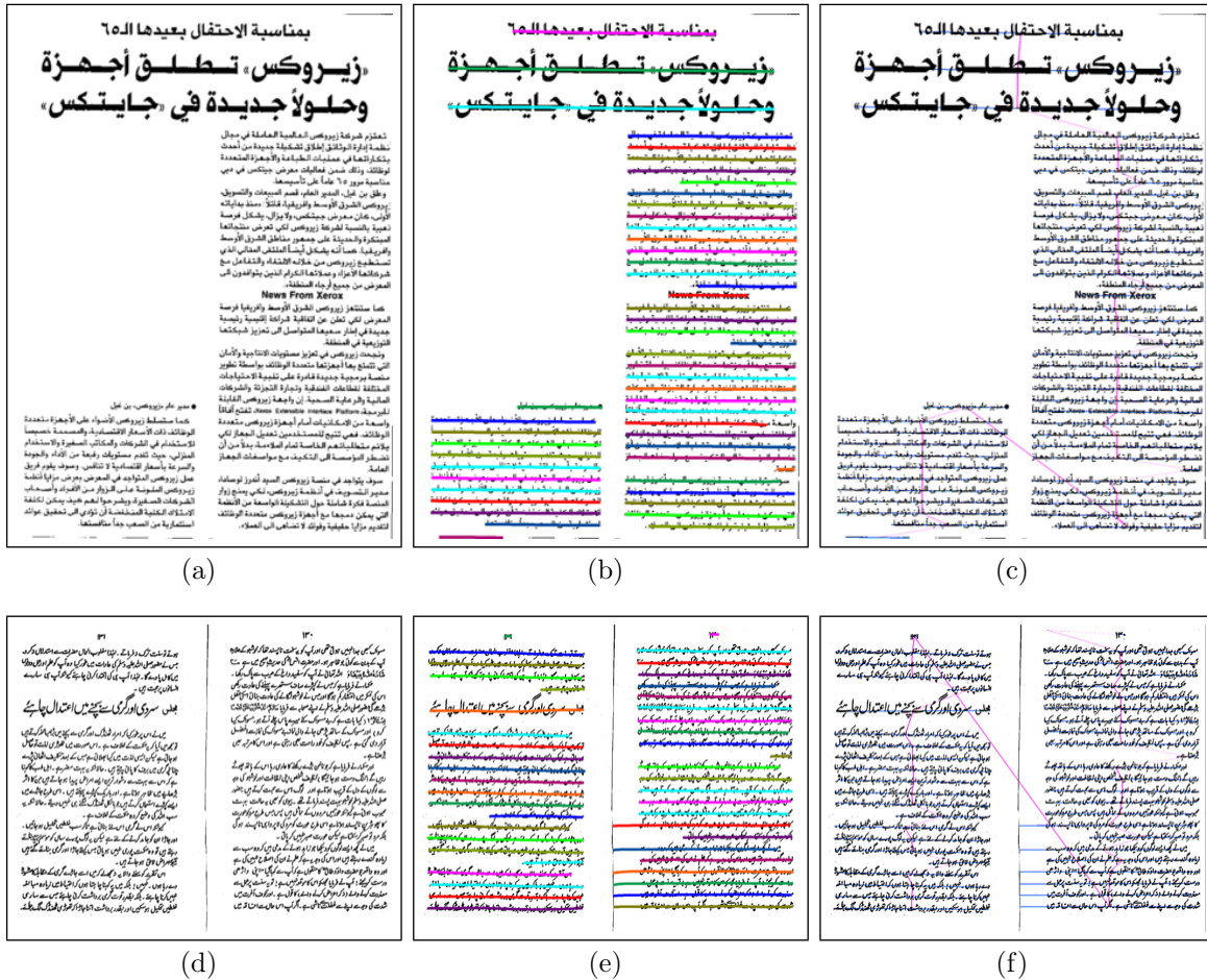
Figure 10.10: Example images illustrating results of reading order for a newspaper and a book page. Thin horizontal lines with different colors indicate detected text line segments, and the magenta lines running down and diagonally across the image indicate reading order.
