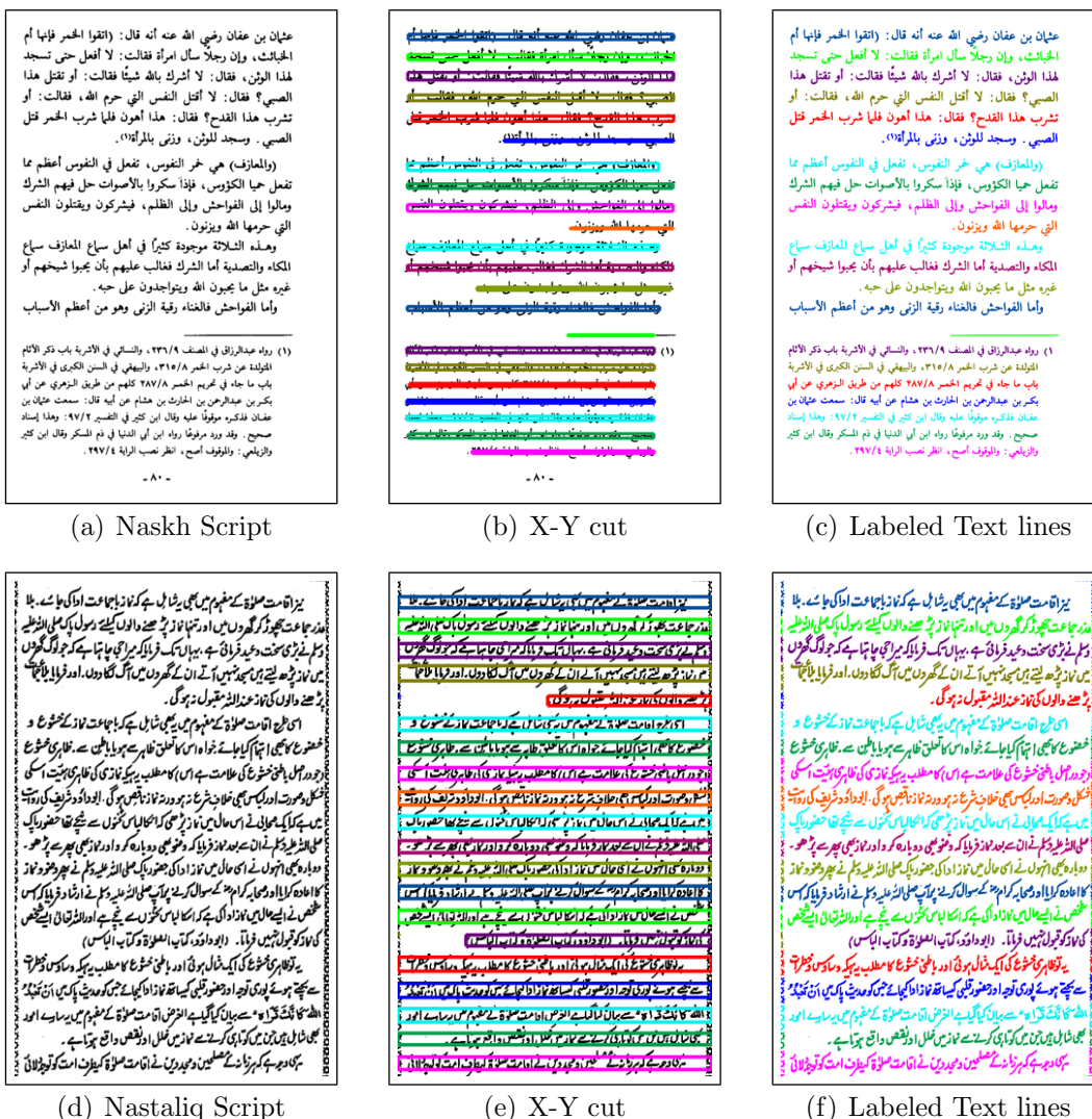
Figure 10.6: The X-Y cut algorithm produces correct text line segmentation results for sample Arabic script document images.
