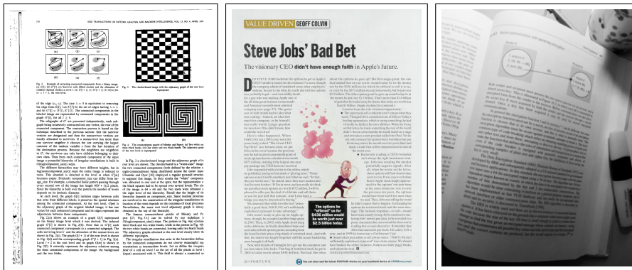
(a) Scanned, Binary, Typewritten Latin Script, Manhattan Layout (b) Scanned, Color, Typewritten Latin Script, Non-Manhattan Layout (c) Camera-Captured, Typewritten Latin Script, Warped Document
