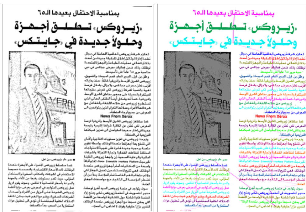
Figure 10.3: A sample newspaper image printed in Arabic Naskh script and its corresponding layout analysis result: gray-region represents non-text components, color-coded labeling represent segmented text lines and magenta-line shows text lines reading order. [Note: left image has been taken from the website [IJM].]
