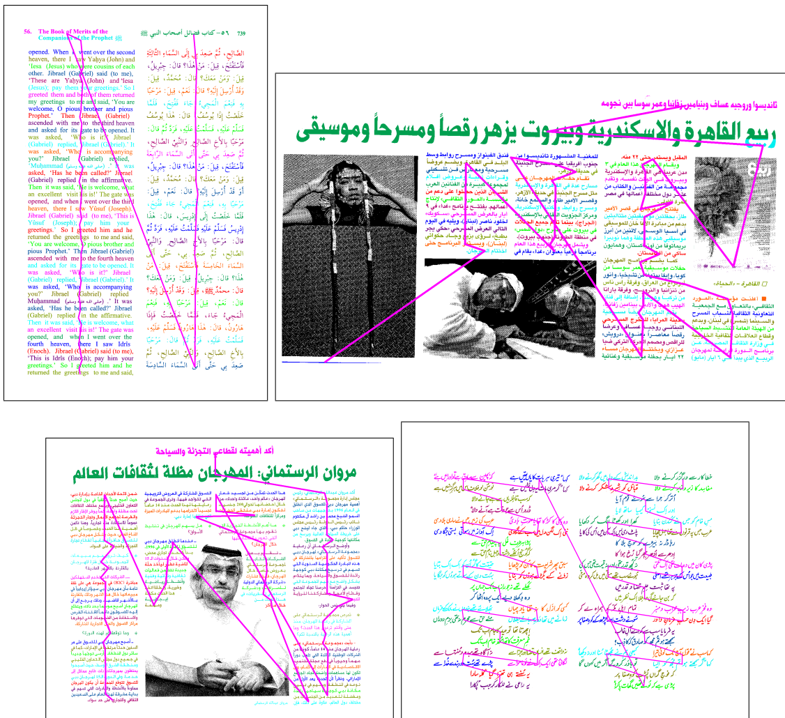
Figure 10.11: Sample images from Arabic and Urdu documents datasets and their corresponding layout analysis results: the black-pixels represents non-text components, the color coded labeling represent extracted text lines and the magenta-line shows reading order of segmented text lines. [top-left] Arabic-English book page; [top-right and bottom-left] Arabic newspapers (these images have been taken from the websites: http://www.alrostanmanigroup.ae and http://www.mawred.org , respectively; [bottom-right] Urdu poetry image.
