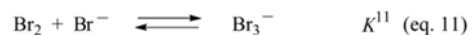
Scheme 17. Equilibria between HOBr, Br 2 , and Br 3 - in H 2 O [ K^{10}=1.45 \times 10^8 \text{ M}^{-2} for H 2 O at 20 °C ( I=0.1 M, pH 2.6–3.8) [145] or 1.04 \times 10^8 \text{ M}^{-2} in H 2 O at 25 °C (pH 1.5) [146]; K^{11}=16.9 \text{ M}^{-1} in H 2 O at 25 °C [147]; 9 \times 10^6 \text{ M}^{-1} in CH 3 CN at 25 °C; 1.5 \times 10^7 \text{ M}^{-1} in DMC at 25 °C].
