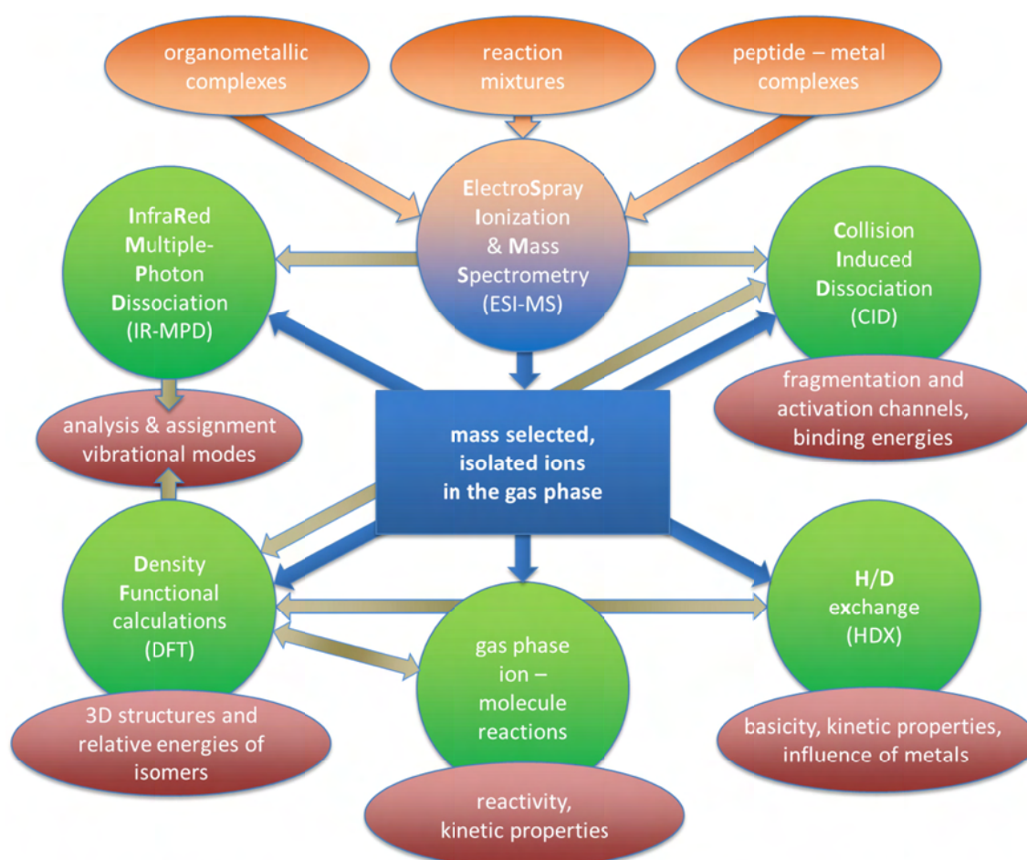
Scheme 1: Liquid samples (orange ovals, top) provide for ionic complexes. Those are transferred to the gas phase (blue square) by electrospray ionization mass spectrometry. Mass selected, isolated ions can be object of different mass spectrometric techniques and density functional theory (green bubbles). Each technique and DFT calculations provide for specific data (wine red ovals). These data can be compared to each other (other arrows).
