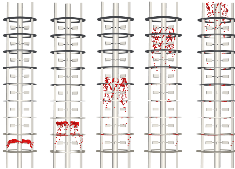
Figure 7.18: Particle flow for the determination of the dispersed phase axial dispersion coefficient at a flow rate of 8 l/h for each phase and 3.8 mm droplets at 100 rpm.
