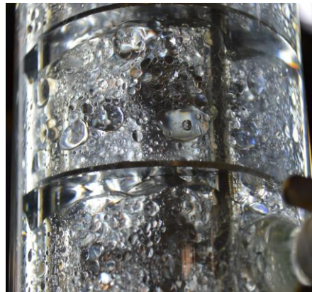
Figure 7.47: Polydispersity due to accumulation of droplets underneath the stators resulting in new droplet dispersion and droplet rise.
