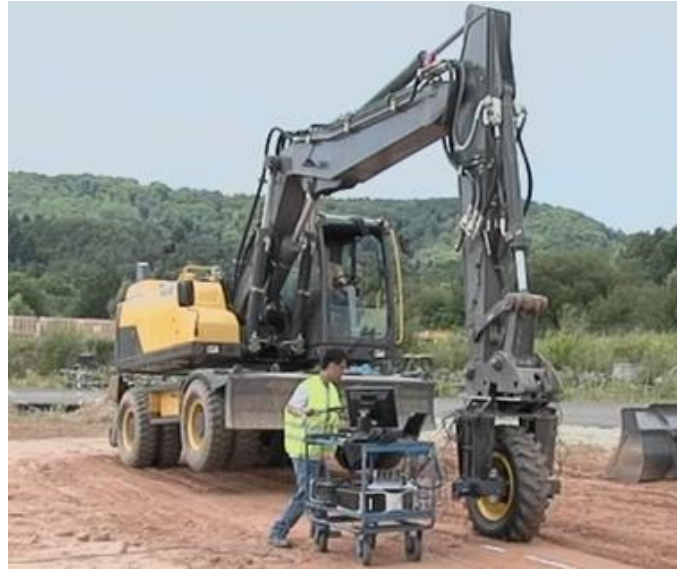
Fig. 6.29: Tire rolling tests
