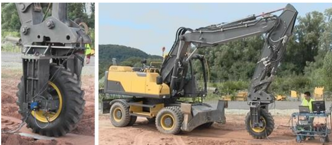
Fig. 6.25: Tire sinking test
