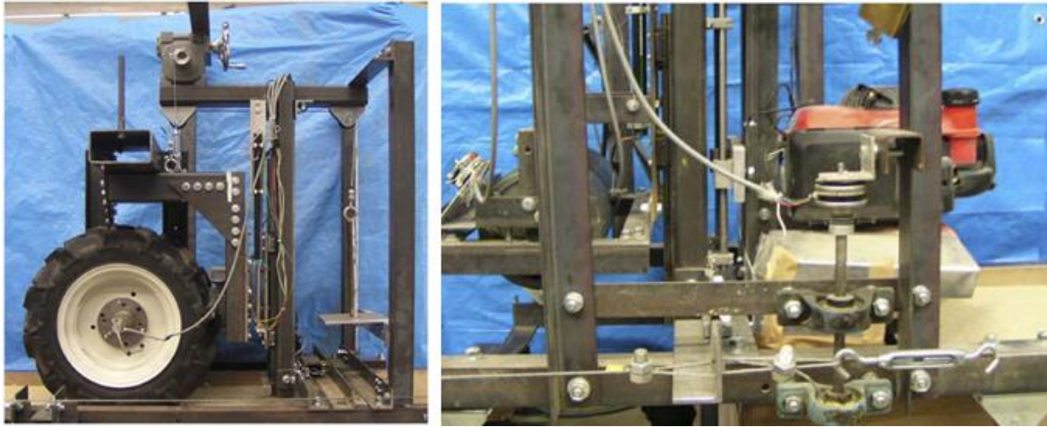
Fig. 2.43: Single wheel tester and a device for soil preparation [115]
