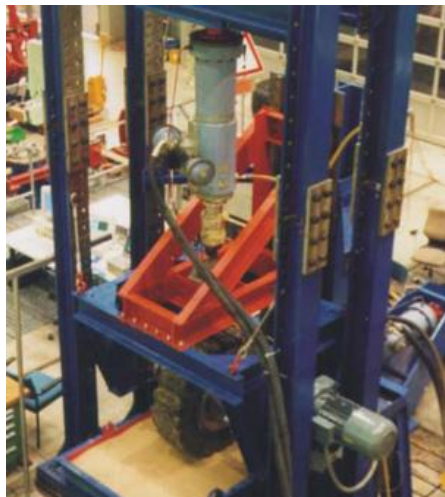
Fig. 2.42: Universal loading-test device [114]
