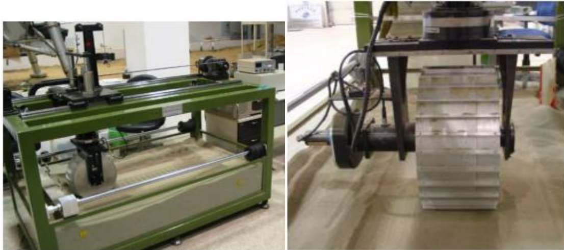
Fig. 2.45: Wheel-soil interaction test-bed [118]
