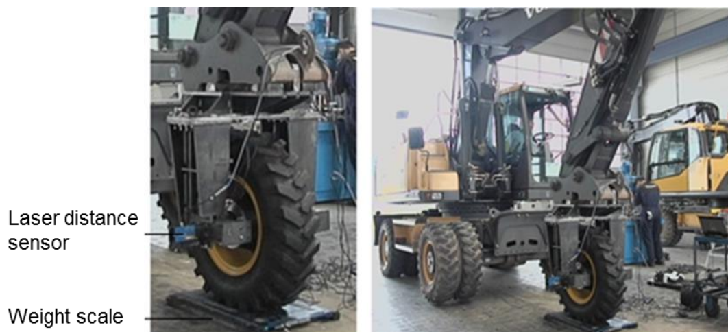
Fig. 6.13: Experiments for the validation of the FE tire model
