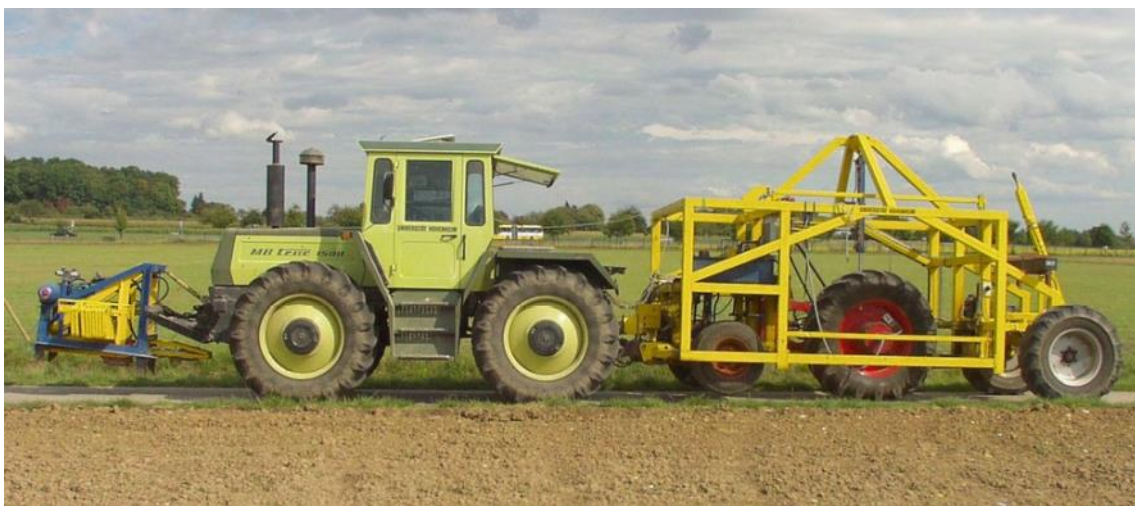
Fig. 2.48: Single wheel tester [122]
