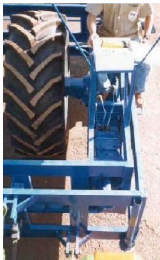
Fig. 2.50: Single wheel tester with mechanical transmission [125]
