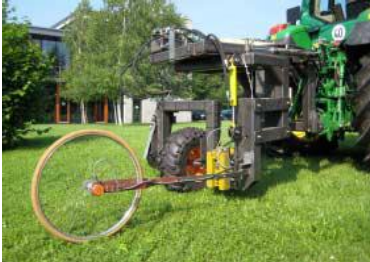
Fig. 2.49: Mobile test rig mounted on the tractor [124]
