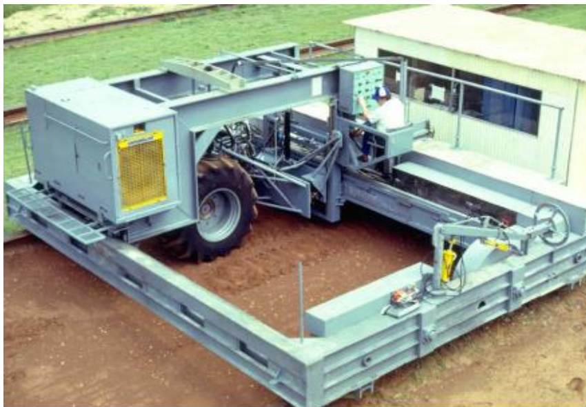
Fig. 2.51: Single wheel Traction Research Vehicle [128]
