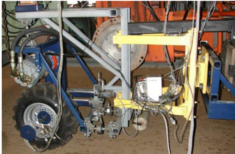
Fig. 2.52: All-Terrain Vehicle tire tester [128]
