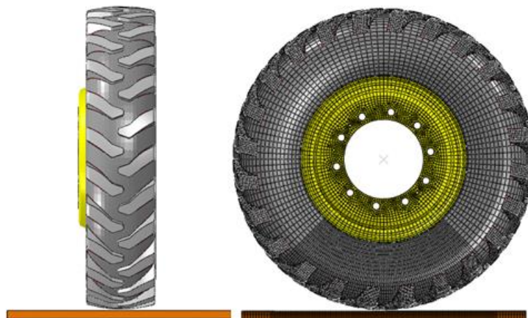
Fig. 5.22: FE model for the tire loading simulation
