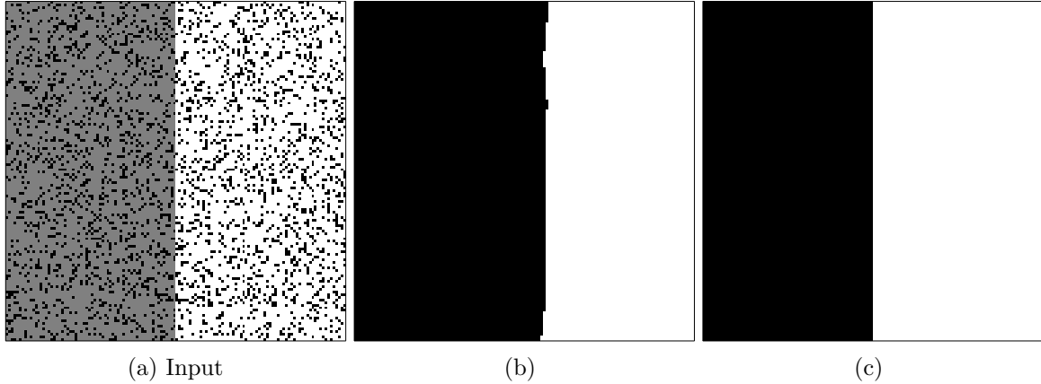
Figure 2.24.: Segmentation of a synthetic image with 20% data missing from [79]. \gamma = 1.5 , \lambda = 3 . a) Input image with 20% data missing. b) Result of STVcM. c) Result of TVcM and ACS.
