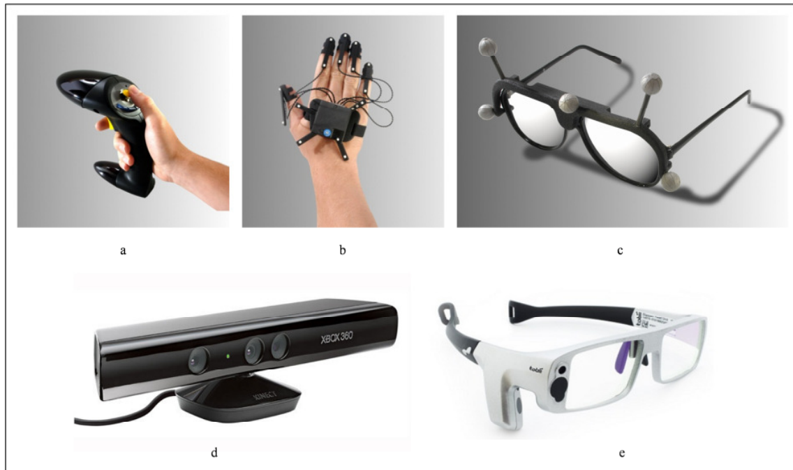
Figure 16: Fly stick (a), finger tracker (b) and 3D glasses with markers from A.R:T., gesture tracker (d) from Microsoft and eye tracker (e) from Tobi
