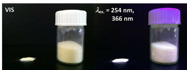
Fig. 8. CIE 1931 chromaticity diagram showing the coordinates of colored and white light emitting fluorogels. Important reference points on the black-body-curve are A (tungsten at 2856 K), B (direct sunlight, 4870 K), C (overcast sunlight, 6770 K) and E (point of equal energy). The emission of fluorogel W-1 under UV light (right) compared to normal light (left) is illustrated by the pictures below the diagram.
