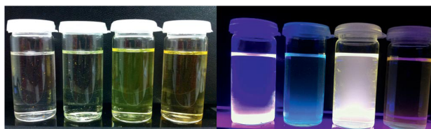
Figure 5. Appearance of (trimethoxysilylthienyl)silane solutions in DCM under normal and UV light ( \lambda_{\text{ex}} = 254/366 \text{ nm} ; from left to right: 6d , 13d , 16d , and 11d ).
