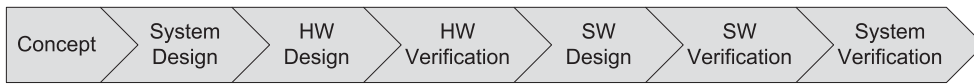
Figure 1.2.: Conventional system design flow (according to [CAT09]). The design flow consists of a sequence of design phases each depending on the outcome of the previous design phase.
