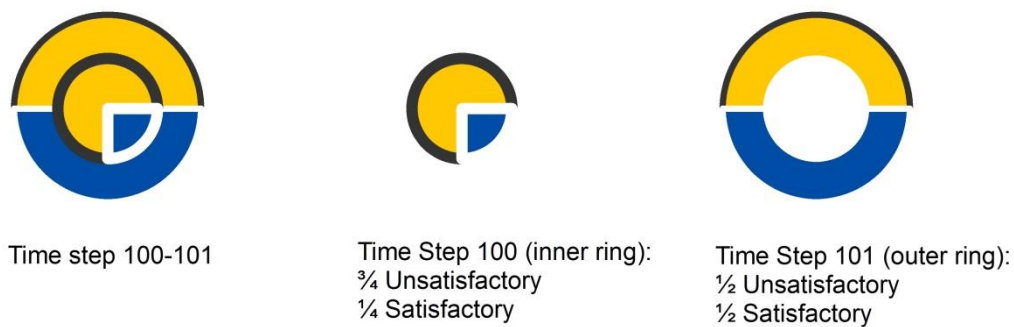
Figure 5.3 Multiple values of a nodal pressure variable are represented as circle view, which was first proposed by Keim et al. (2004).
