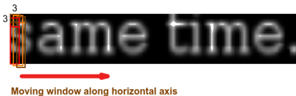
Figure 2.4: Example of sliding window approach: The text line image to be analyzed is shown with overlapping windows and overlapping cells in horizontal and vertical directions. Features are computed from each overlapping (3 x 3) cell, from top to bottom, in every analysis window.
