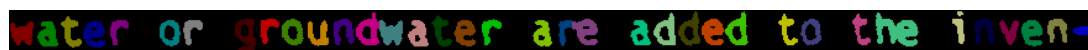
Figure 4.3: Output of character segmentation algorithm in color coded format. Pixels of each segmented character are assigned a unique intensity value and each segmented character is represented by a different color code.
