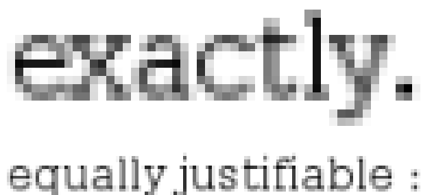
Figure 2.1: Example screen-rendered text images. Character segmentation is difficult due to touching characters and anti-aliasing.
