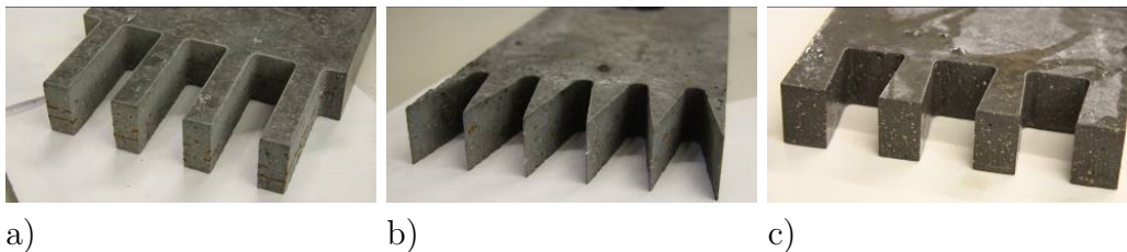
Figure 5.1: Test joint geometries: a) rectangular teeth, b) triangular teeth, c) undercut geometry.
