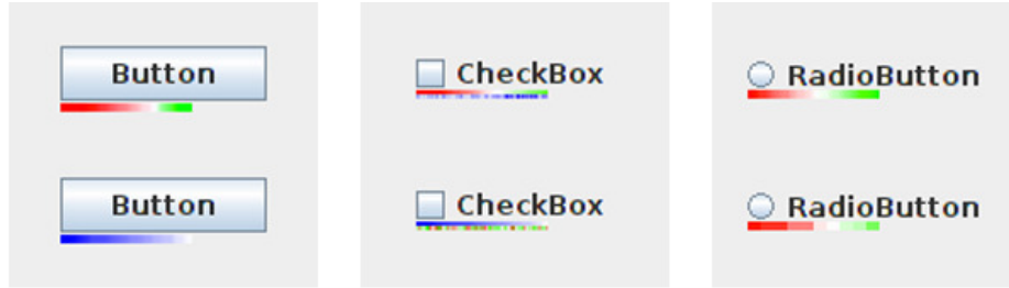
Figure 4.27: Different representations of EmotionScents: Two buttons with their corresponding emotion scent representations for valence (top-left) and arousal (bottom-left). Two check boxes with the valence and arousal EmotionScents displayed in parallel. Depending on the sort priority (i.e., based on valence intensity (top-center) or arousal intensity (bottom-center)), the position of the segments in the second dimension are established by their correspondence to the sorted ones. Two radio buttons presenting their EmotionScents encoding valence (right). The top bar includes over 50 separate EEG readings, thus resulting in over 50 segments that—depending on the interface—can have a width of under one pixel, resulting in a smooth transition between colors and suggesting a high number of emotional readings for that particular widget. For the bottom bar the segments are more visible, as they encode only 10 EEG readings, resulting in wider segments (i.e., larger x values).
