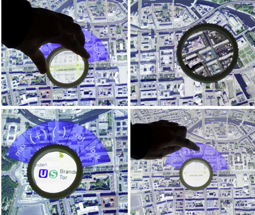
Figure 5.9: An example of TangibleRings enabled interaction: (top-left) the rotation of the ring controls the opacity of the information inside the ring; (top-right) locked view displaced and given to another user to inspect; (bottom) the zoom factor can be changed by using the ring menu or by rotating the ring after selecting 'zoom' as the new control parameter.
