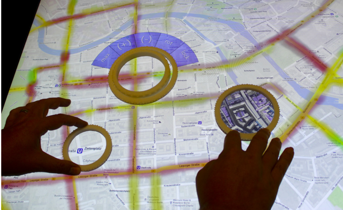
Figure 5.1: TangibleRings in a map-based application, each ring controls different information layers. In this example, the single rings effect only their corresponding lenses, while manipulating the nested rings influences the view on the entire screen.
