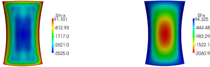
Figure 6.12: Membrane S_{m-x} , bending S_{f-x} stress resultants in the x-direction for Scordelis Lo Roof
