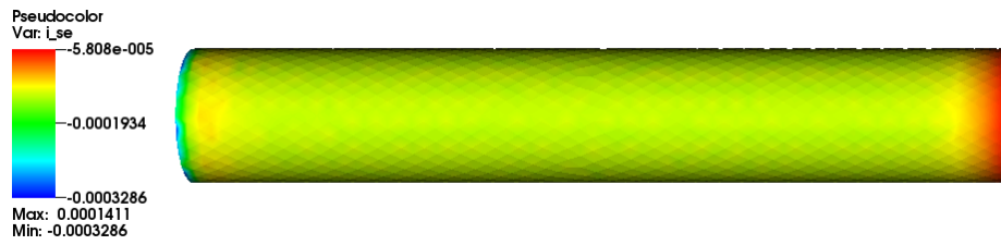
Figure 4.10: Value of i_{se} in a cylindrical particle after 1000s for 1C current
