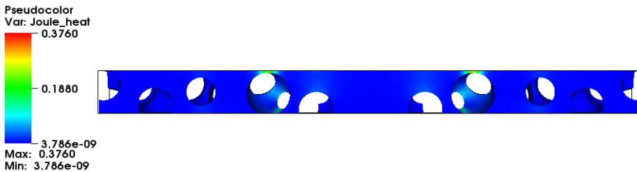
Figure 3.24: Joule heat ( \frac{J}{cm^3s} ) in the electrolyte in the last time step for 2C charging rate for the electrodes with spherical particles
