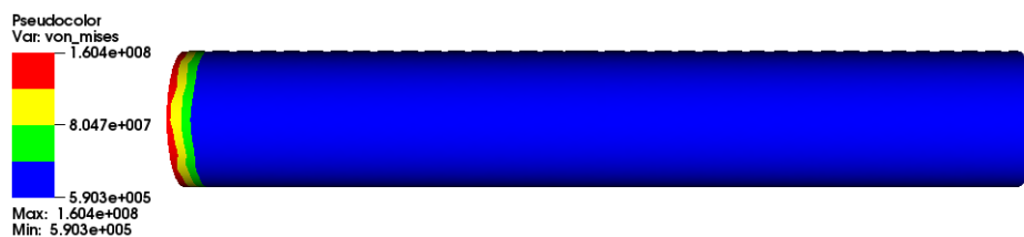
Figure 4.16: Von Mises stress (Pa) in a cylindrical particle using the full electrochemical model after 1000s for 1C current
