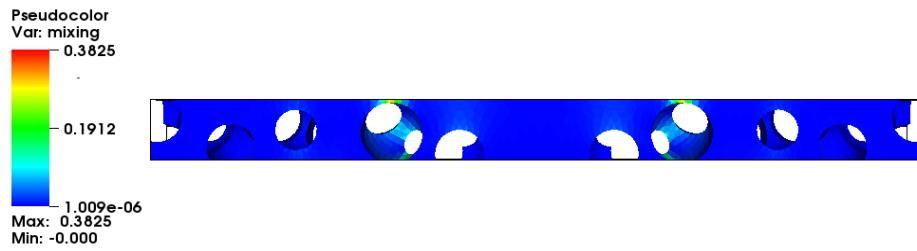
Figure 3.26: Mixing heat ( \frac{J}{cm^3s} ) in the electrolyte in the last time step for 2C charging rate for the electrodes with spherical particles
