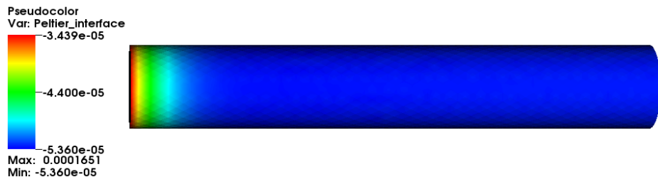
Figure 3.28: The Peltier coefficient term ( \frac{J}{cm^2s} ) at the cathode interface for the cylindrical particles
