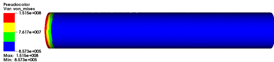
Figure 4.15: Von Mises stress (Pa) in a cylindrical particle using the pure diffusion model after 1000s for 1C current
