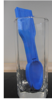
Figure 7.3.1.: Lab-on-spoon for impedance spectroscopy measurement using MEMS switches
