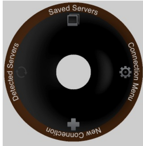
FIGURE 5.1: The general design of the menu, in this example for four menu items, all with a descriptive name and an icon.
