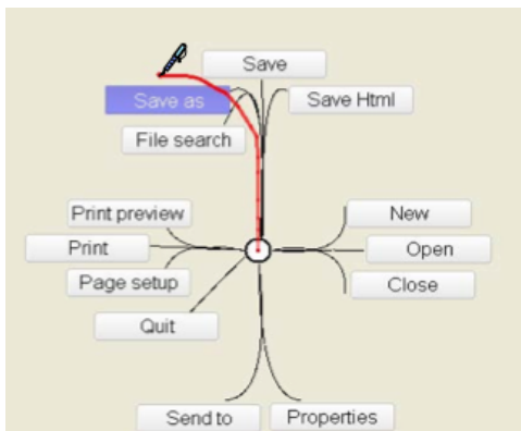
FIGURE 2.4: The design of Flower Menus. Each basic stroke direction (Up, Down, Left, Right) has 3 variations (straight, curved left/right). Courtesy of Bailly and Lecolinet [13]
