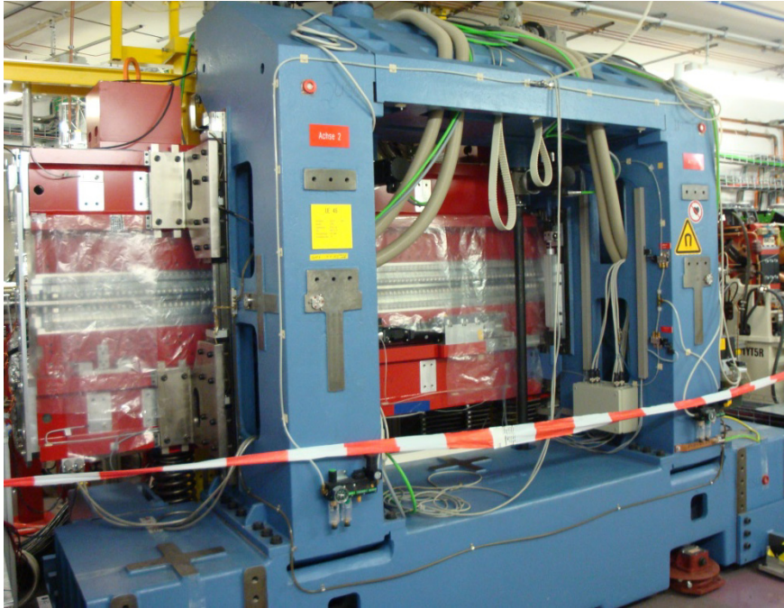
Figure 3.2 Picture of the APPLE2 undulator at the UE52 beamline at the BESSY II synchrotron facility.
