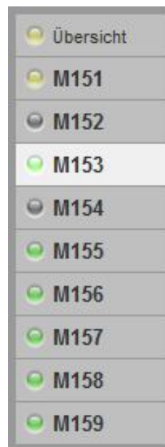
Figure 87 Traffic Light Visualization for Monitoring of eight Extrusion Lines, displaying their Condition States
