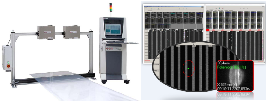
Figure 25 Optical transmission light control system (OCS GmbH) for defect detection in polymer films
