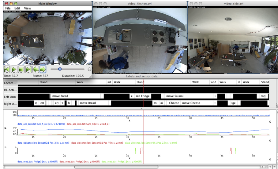
Figure 4.6: A screenshot of the Labeling Tool showing tree parallel video streams (top), four label tracks at different granularity (middle), and plots of several data streams (bottom) around the current master video frame.
